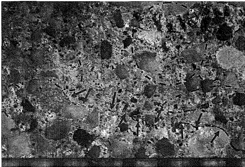
Figure 12. Photomicrograph along the lapped surface of East Parapet core illustrating bleed water channels (red arrows) and small pockets of soft, porous cement paste (within red dashed circles). Scale is in millimeters.
