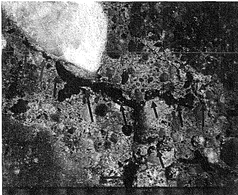
Figure 11. Photomicrograph along the lapped surface of East Parapet core showing bleed water channels and bleed water induced gaps (red arrows). Scale is in millimeters.
