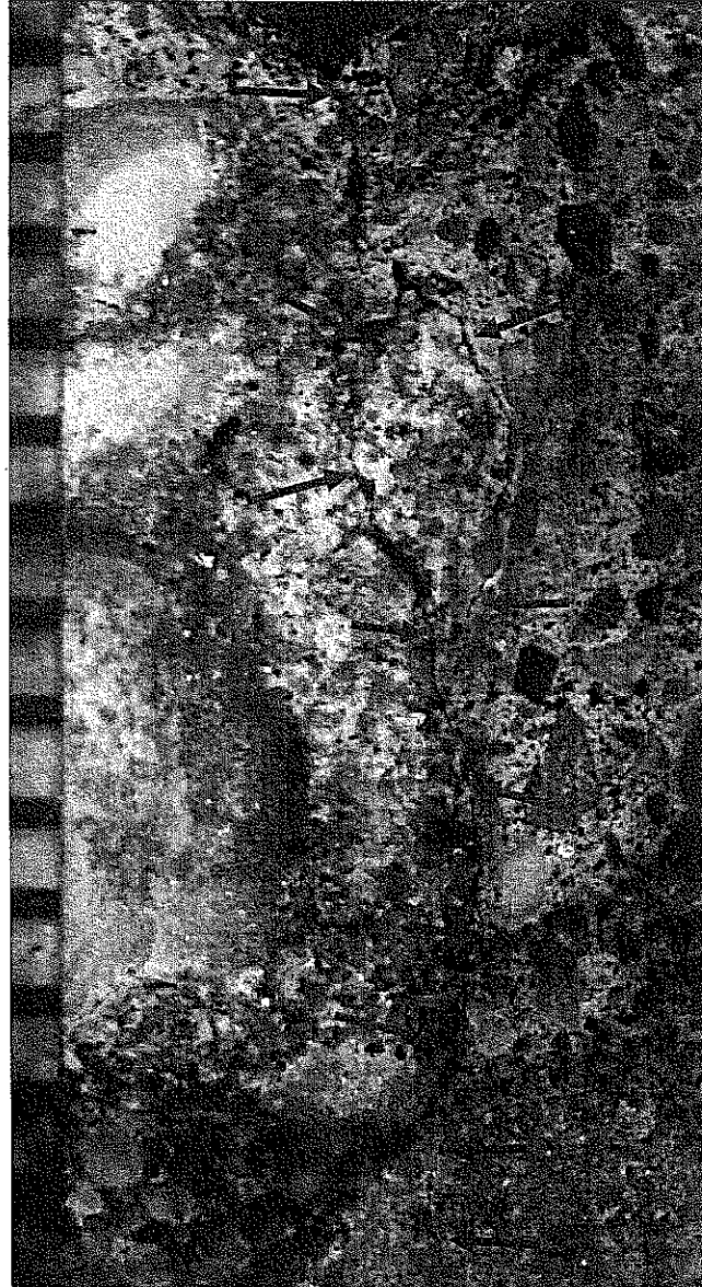
Figure 5. Photomicrograph along the lapped surface of the West Parapet core at and just below the outer surface (at top of photo). Red arrows point to a fine, vertical, microcrack extending from the outer surface to a depth of 12 mm (0.47 in.) where it abruptly terminates in a coarse aggregate particle. The microcrack passes around aggregate particles, suggesting the crack formed before significant development of bond between the cement paste and aggregate. The microcrack appears due to minor drying shrinkage. Scale is in millimeters.
